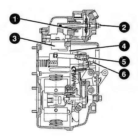
\* Lug cam with torque control
